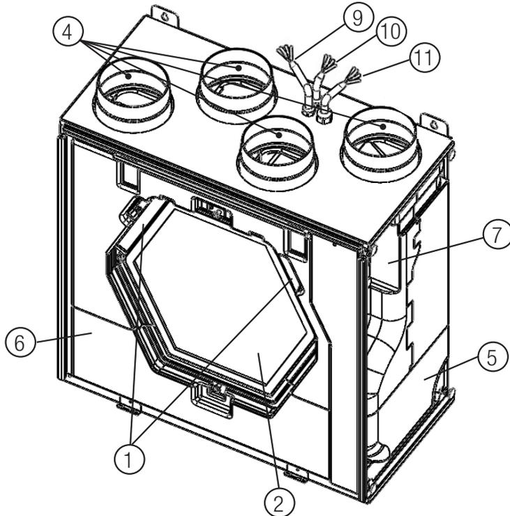
Fig. 8.a SITALI CXVA 280 S1 internal components
