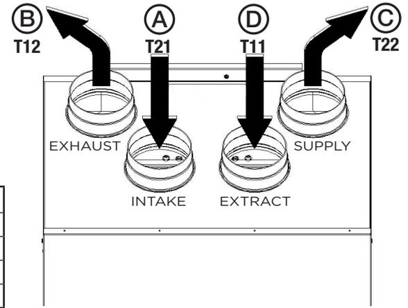
Fig. 7.b SITALI CXVA 400 e SITALI CXVA 550 temperature probes.
