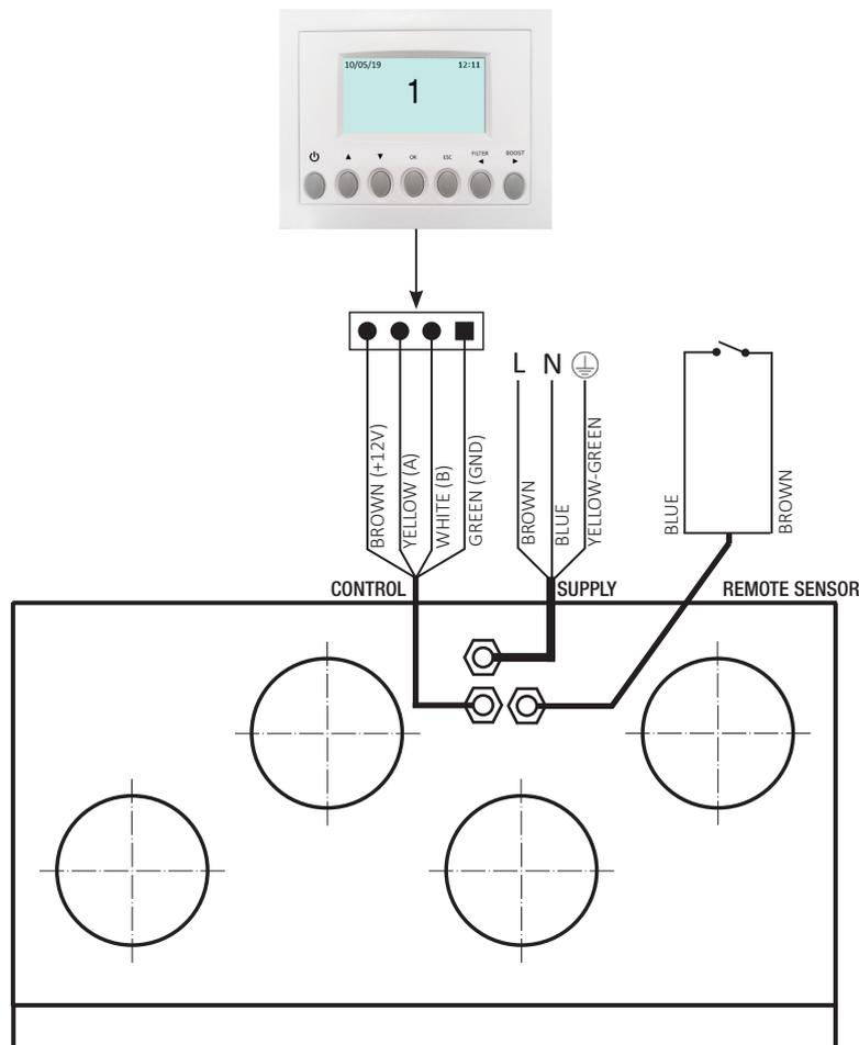
**Fig. 5.p** Electric connections
