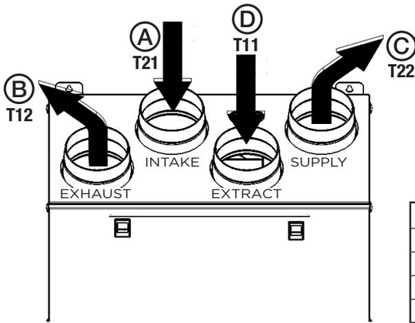
Fig. 7.a SITALI CXVA 280 S1 temperature probes.
